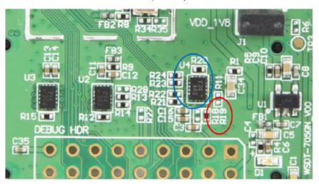
Figure 13. Resistors to Change the Direction of the PCM
