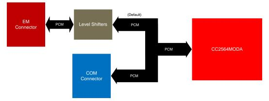
Figure 12. PCM Connector Configuration
