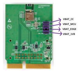
Figure 8. Jumper Configurations
