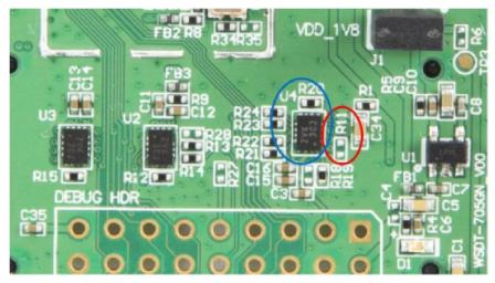
Figure 14. R11 DNI to Enable Audio Features
