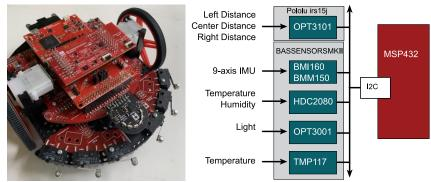
Figure 1. RSLK with the Pololu OPT3101 Time of Flight module used to measure distance, and the TI BP-BASSENSORSMKII Boosterpack used to measure acceleration, rotation, magnetic field, temperature, humidity, and light intensity.
