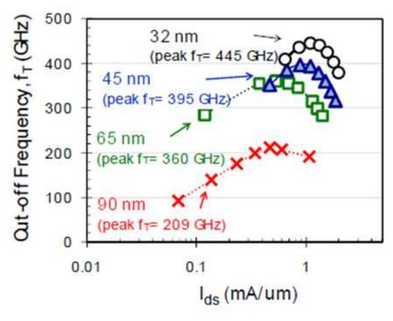
Figure 1. Scaling Trends of  $f_T$  in CMOS
