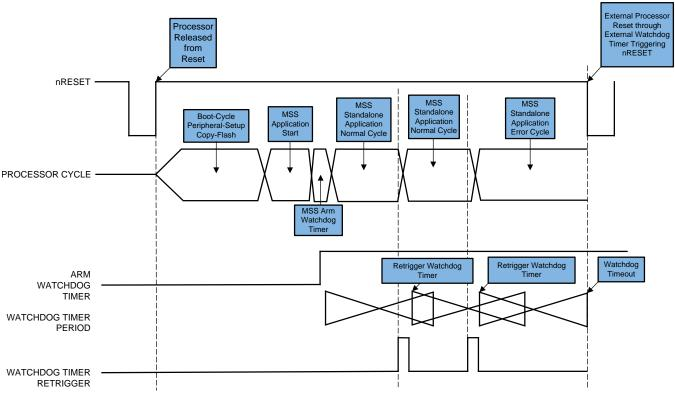
Figure 2. Radar Sensor With External Watchdog Timer
