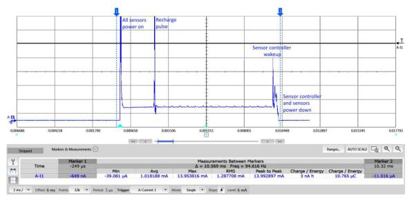
Figure 5. Lazy Sensor Sequencing – All Sensors Powered at Same Time
