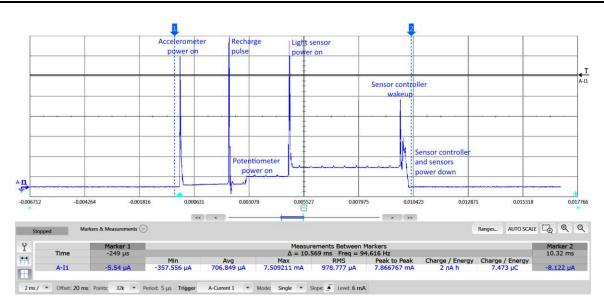
Figure 4. Full Sensor Sequencing Using the CC2642R1 Sensor Controller
