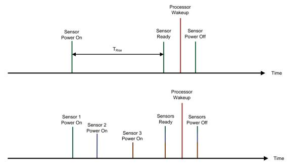
Figure 1. Sensor Sequencing With One and Multiple Sensors
