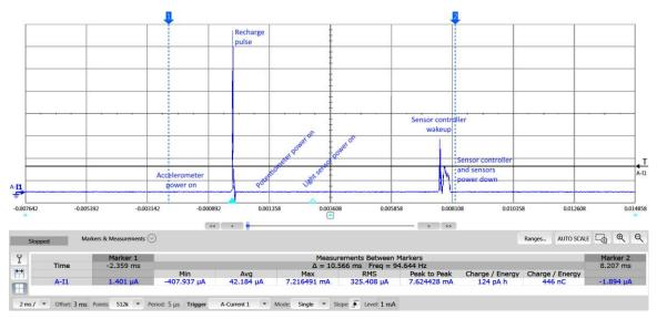
Figure 3. Full Sensor Sequencing Using CC2642R1 Sensor Controller Without Sensors Connected
