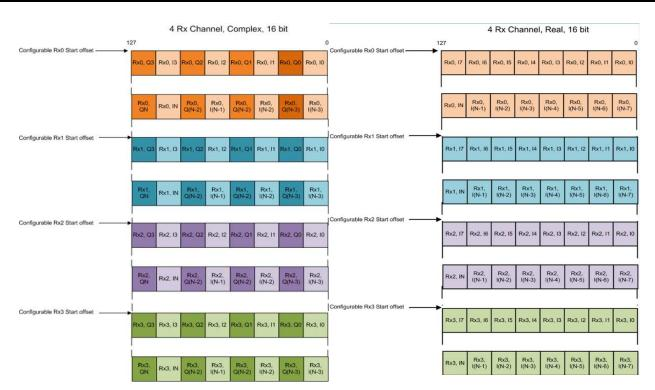
Figure 4. Non-Interleaved Mode of Storage
