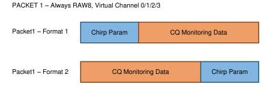
Figure 24. Packet 1 - Configurable Formats
