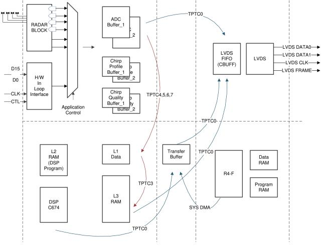
Figure 1. Typical Data Flow in AWR16xx Devices
