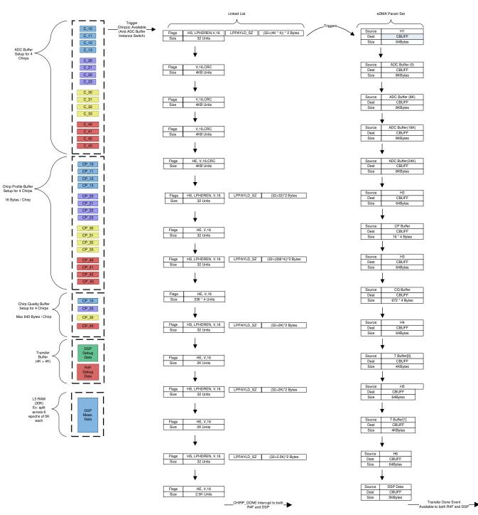
Figure 25. Data Transfer @ Chirp Periodicity
