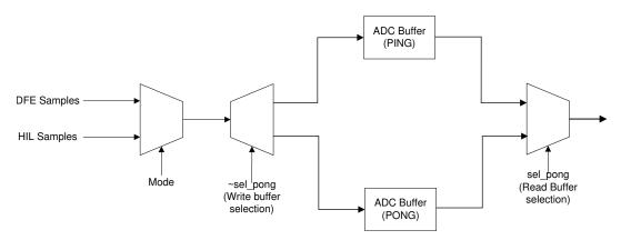
Figure 2. ADC Buffer Write Sources
