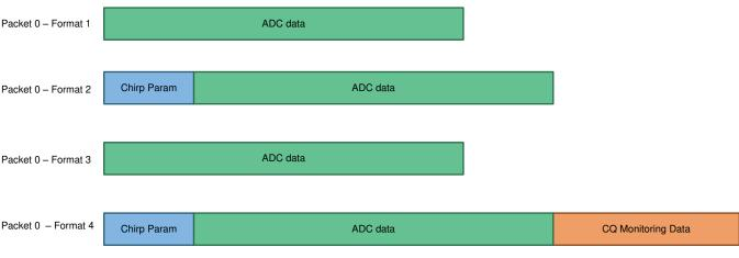
Figure 23. Packet 0 - Configurable Formats
