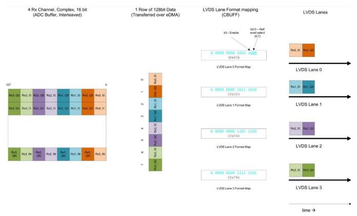
Figure 22. LVDS Format Mapping - Interleaved Mode
