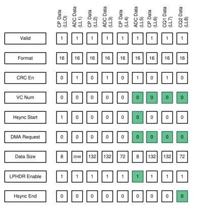
Figure 18. Linked List Configuration - Multiple Packets
