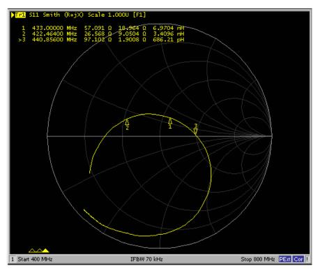
Figure 9. Matching of the Antenna With ANT1 and ANT2 Components
