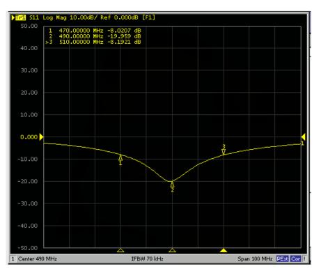
Figure 10. Return Loss With ANT1 and ANT2 Components
