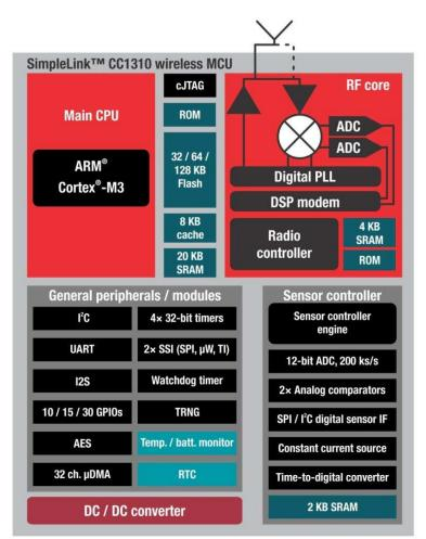
Figure 2. CC1310 Block Diagram
