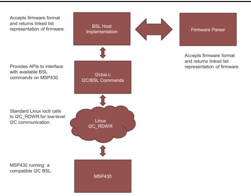
Figure 1. Overall I<sup>2</sup>C BSL Update Block Diagram
