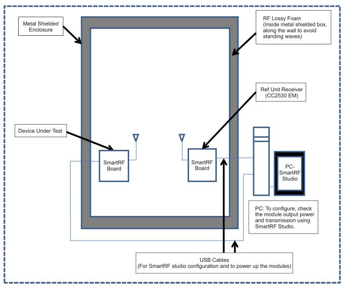
Figure 1. Suggestion 1: Setup Used in Production Line
