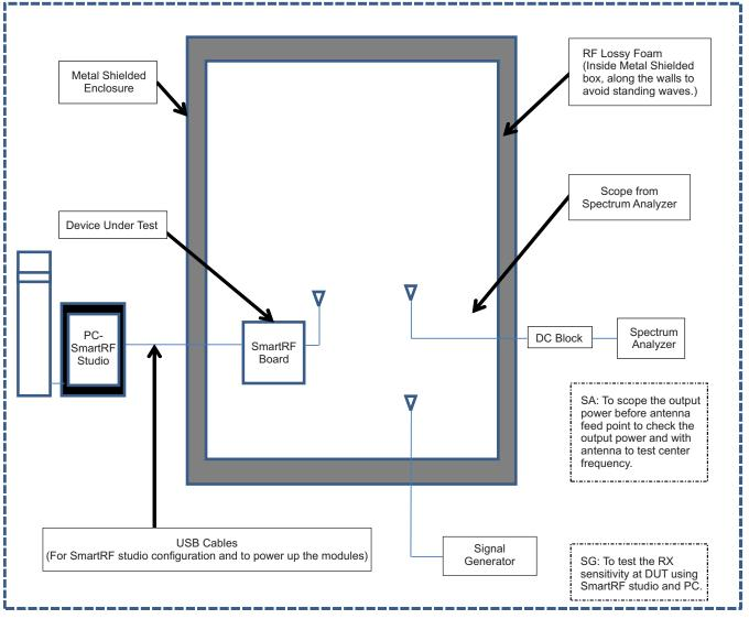
Figure 2. Suggestion 2: Setup Used in Production Line
