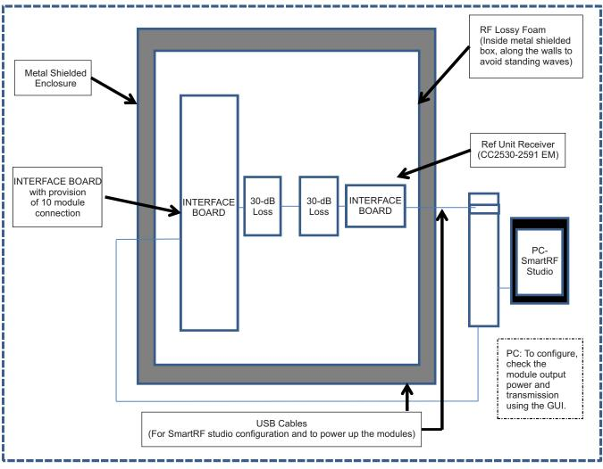
Figure 3. Suggestion 3: Setup to be Used in Production Line
