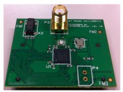
Figure 2. Photo of TDK filter solution
