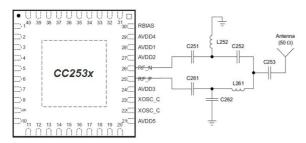
Figure 3. Discrete ref design for the CC253x
