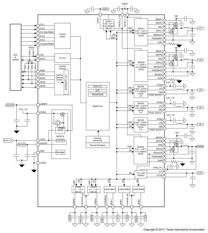
Figure 2. TPS650860 Example Block Diagram
