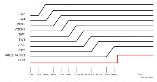
Figure 4. Timing Diagram of Power Rails for MC13982 (Source: Freescale AN4053.pdf Application Note)
