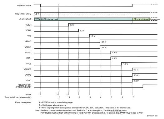
Figure 3. Power-Up Timing Diagram
