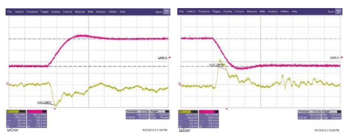
Figure 7. Single-Phase Load-Step Response 3.3-V Input, 1.8-V Output, 94 µF, Hot
