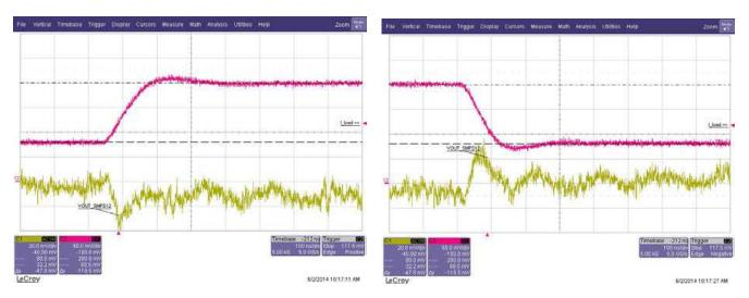
Figure 15. Dual-Phase Load-Step Response 5-V Input, 3.3-V Output, 194  $\mu$ F, Hot
