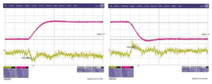
Figure 13. Dual-Phase Load-Step Response 5-V Input, 1.05-V Output, 194 µF, Hot
