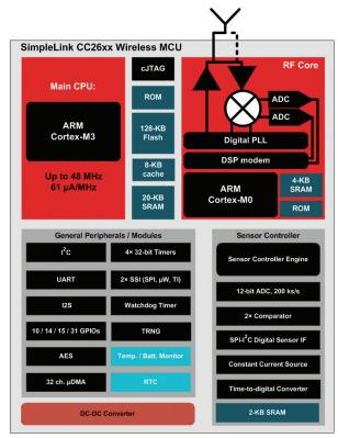
Figure 6. SimpleLink CC26xx wireless MCU functional diagram.
