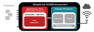
Figure 5. Block diagram of a SimpleLink CC3220 wireless MCU.
