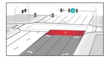
Figure 2. An intersection where traffic radar sensors can be positioned at the stop bar (1) or on the traffic pole (2). Sensors on the traffic pole do not require installation in the road's surface.
