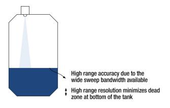
*Figure 1*. High resolution 77 GHz radar improves performance for industrial level sensing.
