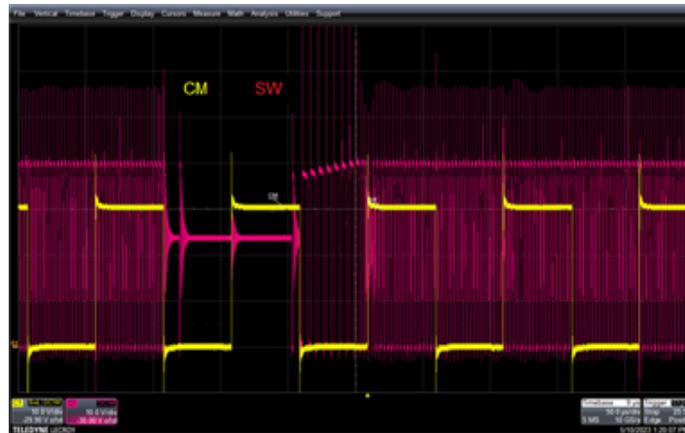
**Figure 3. PSR flyback affected by CMT (vertical: channel 1 = 100 V/div, channel 2 = 10 V/div; horizontal: 50  $\mu$ s/div)**
