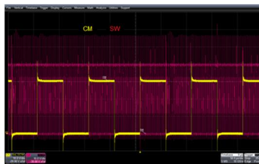
Figure 7. LM5180EVM-S05 performance with CMTI mitigation (vertical: channel 1 = 100 V/div, channel 2 = 10 V/div; horizontal: 50  $\mu$ s/div)
