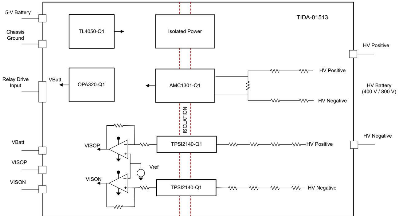
**Figure 5. Leakage measurements reference design block diagram**
