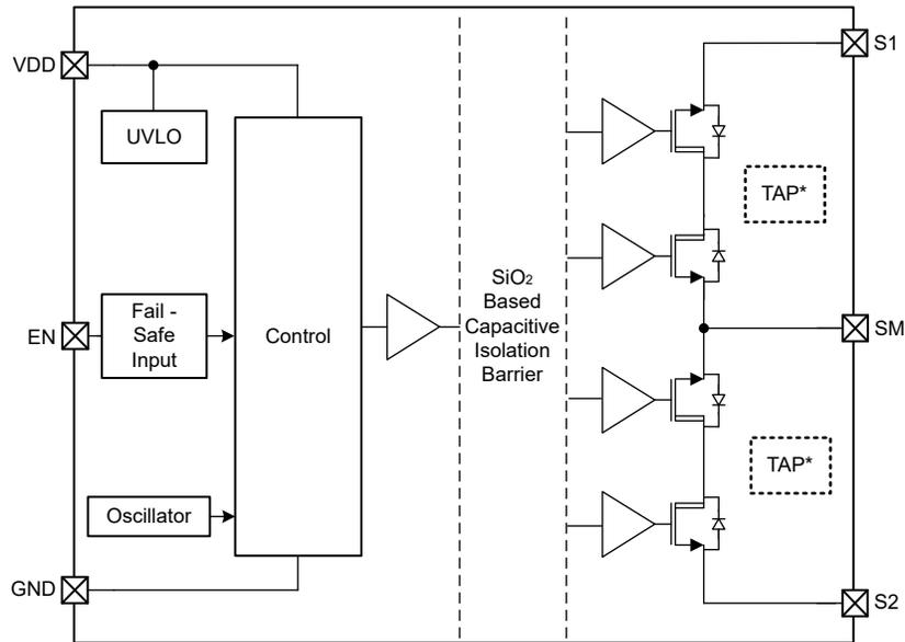
**Figure 3. TPSI2140-Q1 functional block diagram**
