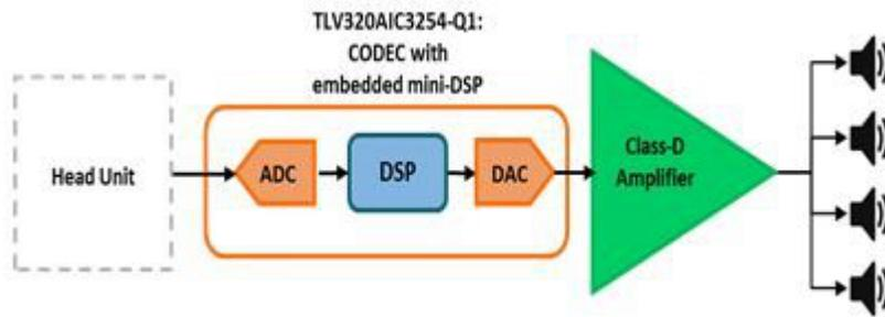
**Figure 2. Mid-end Automotive Amplifier: Integrated Preamplifier with Gain Control and EQ**
