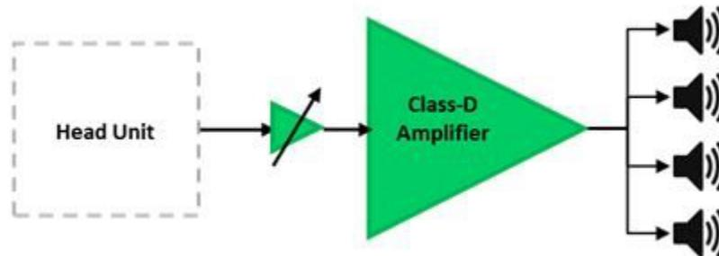
**Figure 1. Low-end Automotive Amplifier: Discrete Preamp and Amplifier**
