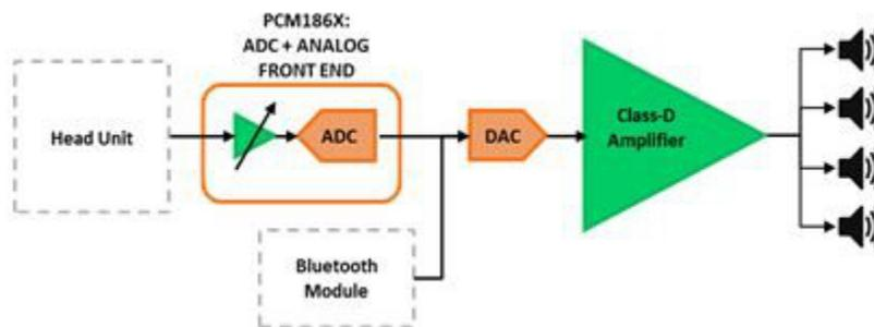
**Figure 3. High-end Automotive Amplifier: Integrated Preamplifier with Analog Gain Control, Crossover and EQ**
