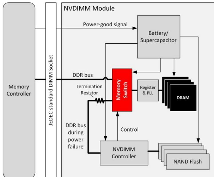
**Figure 1. Using a Memory Switch in NVDIMM Application**
