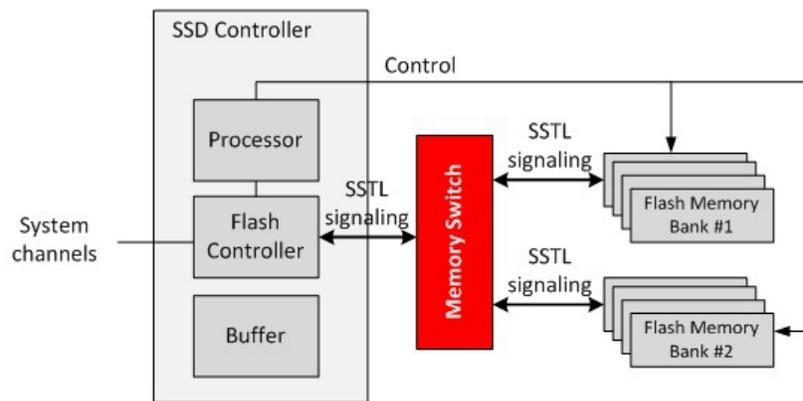
**Figure 2. Using a Memory Switch in Load Isolation Application**
