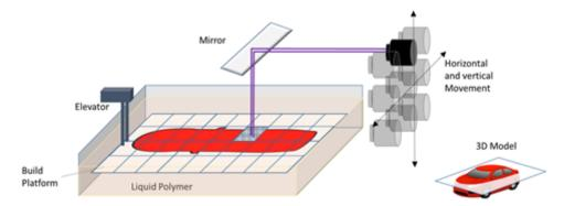
Figure 1. This diagram shows how MOVINGLight® technology is moving the DLP technology projected image over the build area
