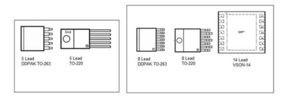
Figure 1. LM2576, LM2596, and LM2676 Regulators
