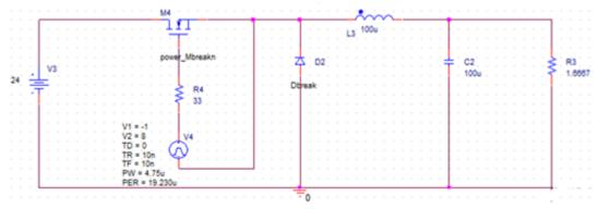
Figure 1. Simple Buck Simulation Schematic
