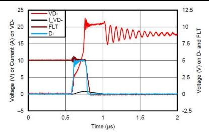
Figure 3. TPD3S714-Q1 Data Switch Short-to-18V Response Waveform
