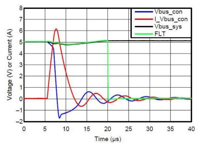
Figure 4. TPD3S714-Q1 V<sub>BUS</sub> Short-to-ground Response Waveform
