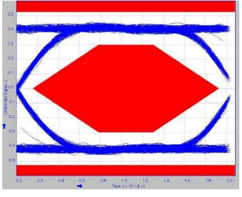
Figure 2. USB 2.0 Eye Diagram with the TPD3S714-Q1
