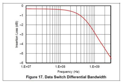
Figure 1. TPD3S714-Q1 Data Switch Differential Bandwidth
