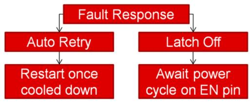
Figure 1. eFuse Fault-response Options (Auto Retry and Latch off)
