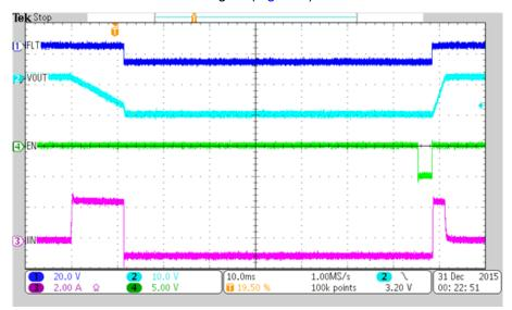
Figure 5. TPS25942L Current-limiter Latch-off Functionality
