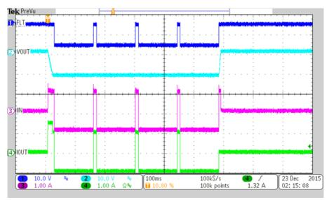
Figure 3. TPS25942A Current Limiting and Auto Retrying
