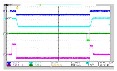
Figure 4. TPS25944L Circuit-breaker Latch-off Functionality
