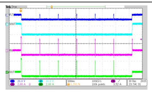
Figure 2. TPS25944A Circuit Breaking and Auto Retrying
