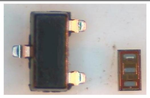
Figure 2. Traditional SOT-23 Package Next to the CSD18541F5 LGA Package
