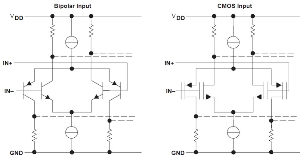
**Figure 2. One Common Input-stage Topology for a Rail-to-rail Input Amplifier Using a Bipolar Junction Transistor (BJT) (Left) or MOSFET (Right)**
