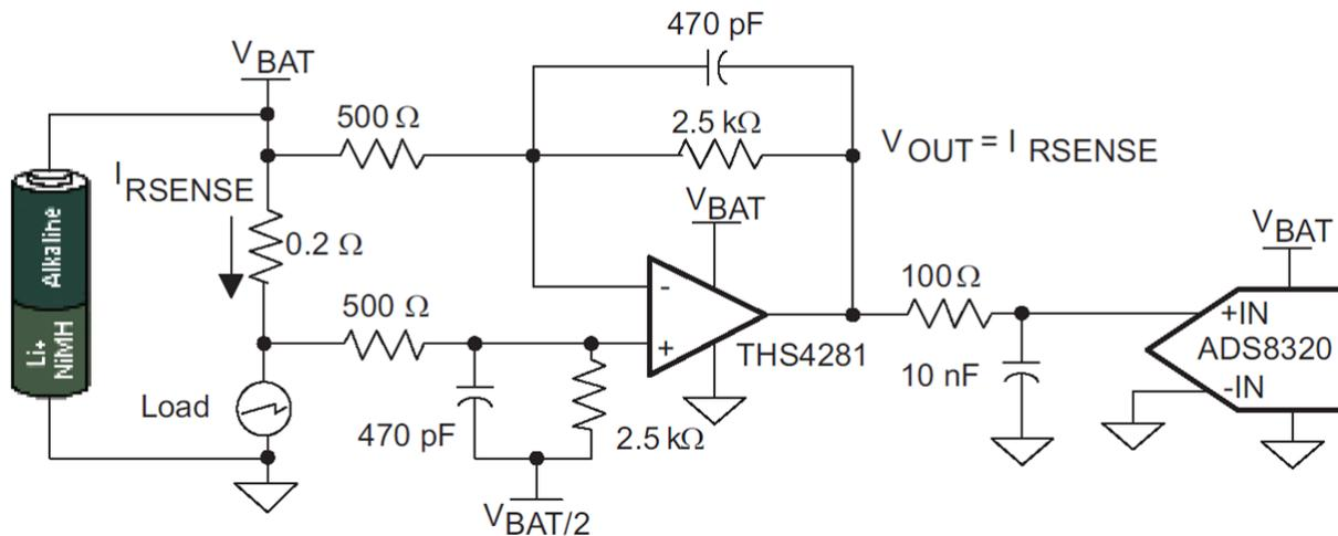
**Figure 1. A Typical High-side Current-sensing Circuit for Battery Systems Using the THS4281**
