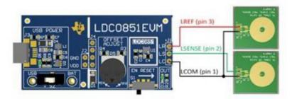
Figure 5. Connecting the Sensor Coils to the LR, LS and LC Terminals of J1
