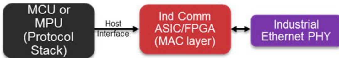
**Figure 1. The traditional way to add industrial Ethernet**
