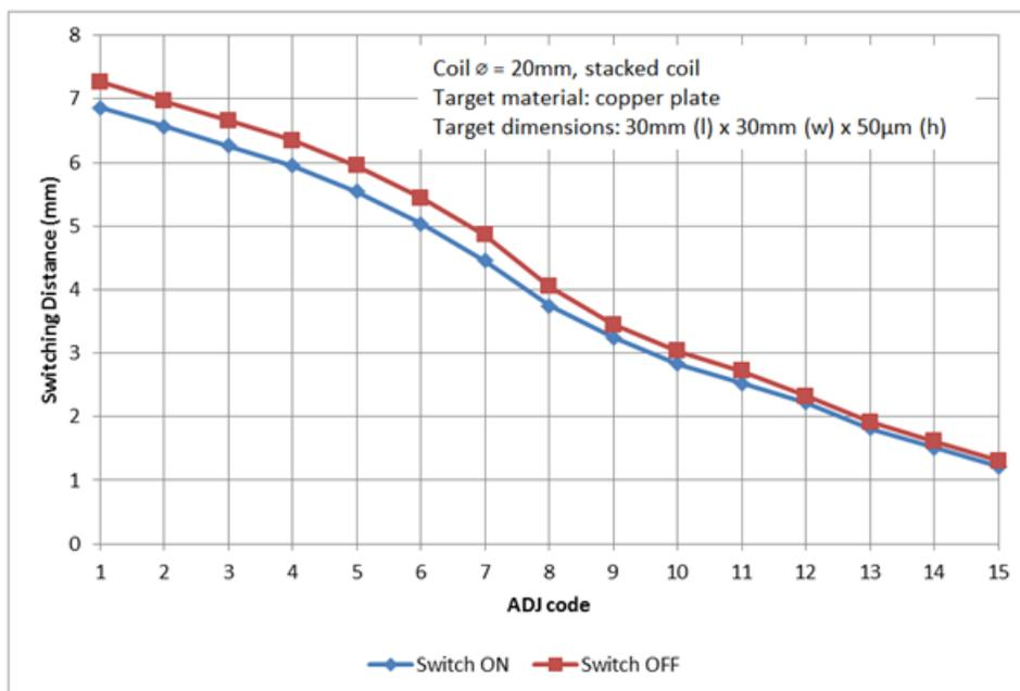
Figure 4. Threshold Set and Release Points
