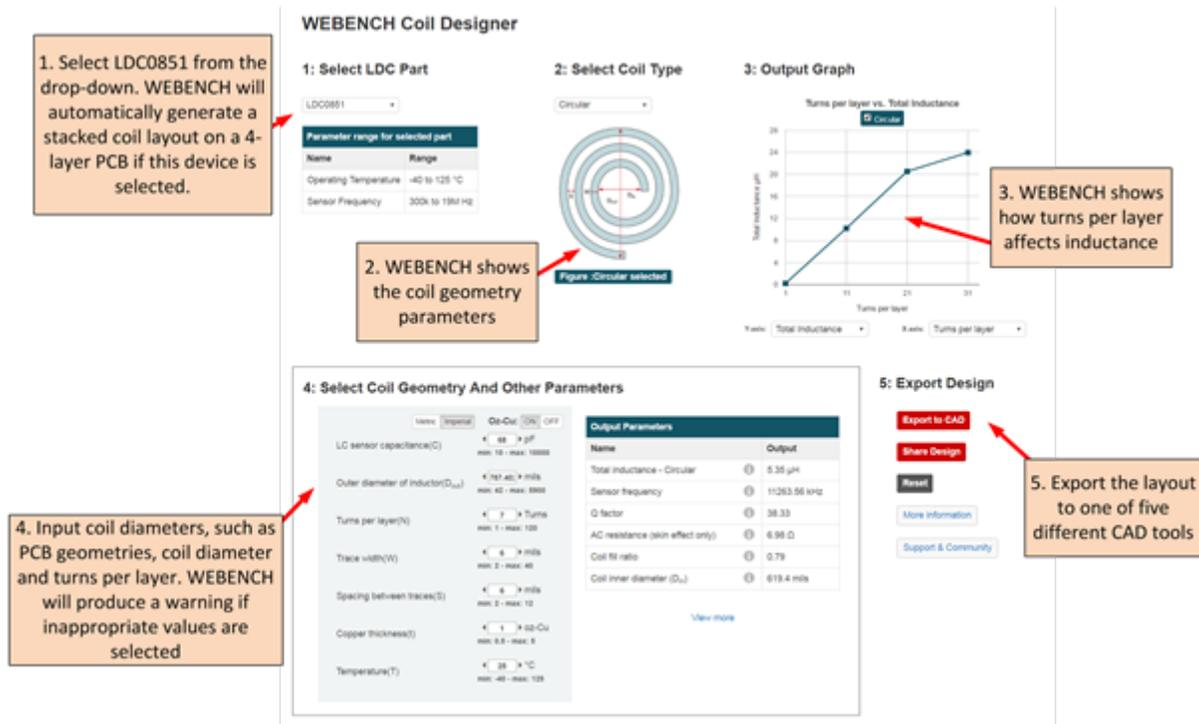
**Figure 2. Five Steps for Designing a Stacked Coil in WEBENCH Coil Designer**
