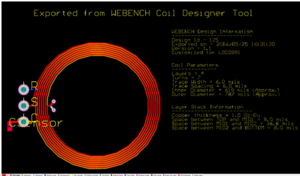
Figure 3. The Finished Coil in Altium Designer Format
