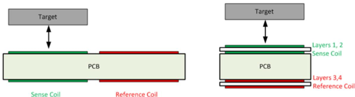
Figure 1. Side-by-side Coil Arrangement (Left) vs. Stacked Coil Arrangement (Right)
