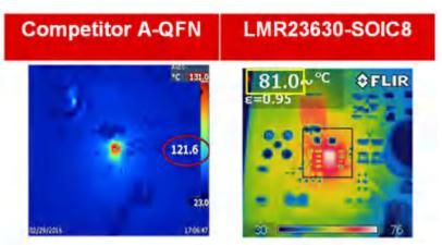
Figure 1. Thermal Images Taken at  $v_{IN}$  = 12V,  $v_{OUT}$  = 5A at 3A, 2MHz
