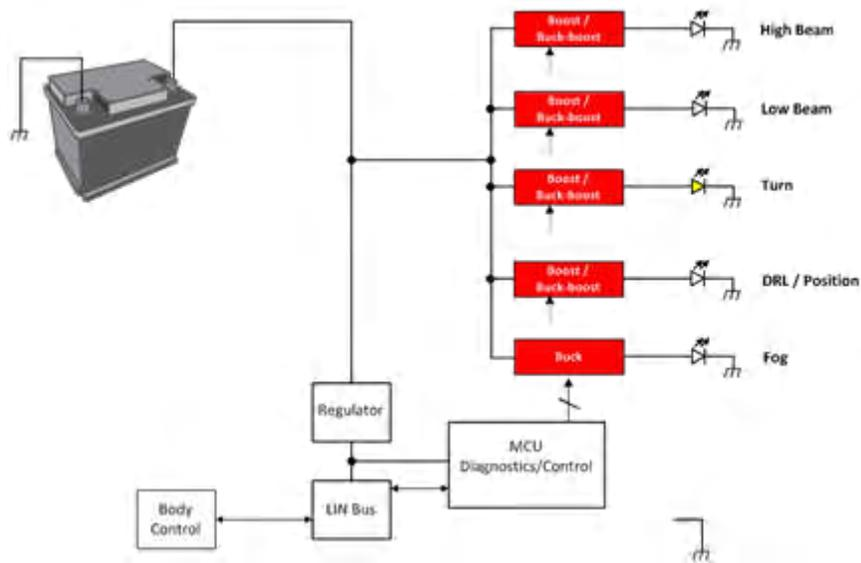
**Figure 1. Single-stage Architecture for Automotive Front Lighting**
