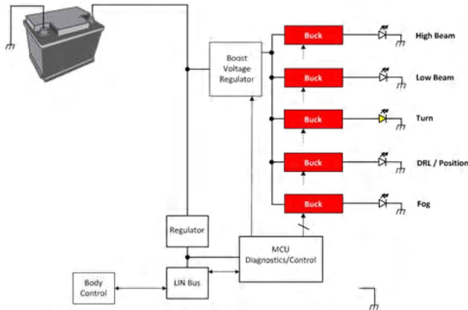
**Figure 2. Two-stage Architecture for Automotive Front Lighting**
