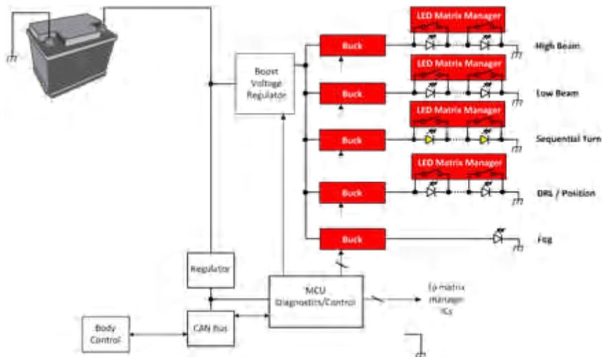
**Figure 3. Adaptive Headlight Based on a Two-stage Architecture with Matrix-manager Devices**
