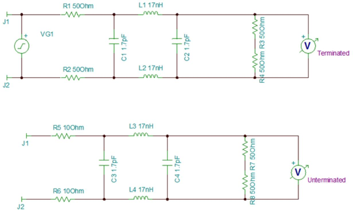
Figure 5. Filters with Different Driving Impedances
