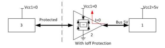
Figure 2. Device with Powered-off Protection
