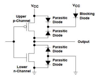
Figure 3. Typical Powered-off Protection Circuit
