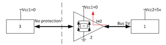
Figure 1. Device without Powered-off Protection
