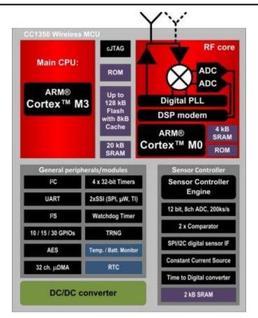
Figure 1. Block Diagram of the SimpleLink Dual-band CC1350 Wireless MCU
