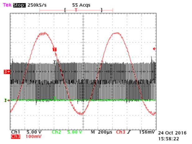
Figure 2. Measuring Phase Current Amidst Fast Common-mode Transients
