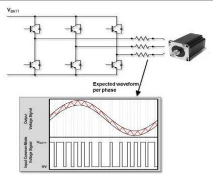
Figure 3. Expected Voltage Waveform Due to Enhanced PWM Rejection
