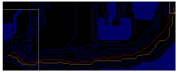
Figure 2. Differential Routing Feedback Showing Output Voltage Feedback (Red), Ground Feedback (Orange) and Package Outline (White)
