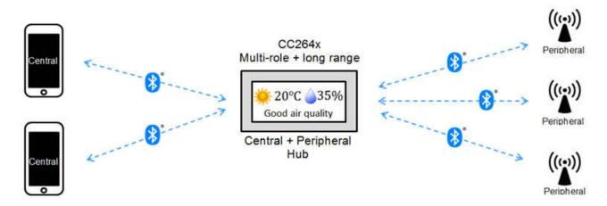
Figure 1. Home Air Quality Sensing System Using Multi-role
