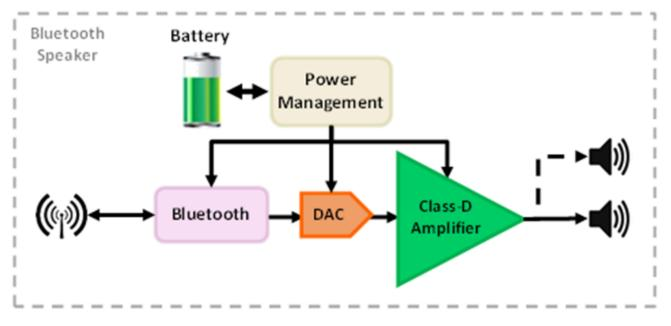
Figure 1. Bluetooth Speaker Block Diagram
