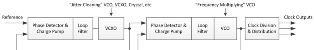
Figure 2. Dual-loop Jitter Cleaner
