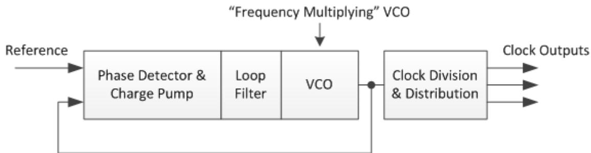
Figure 1. Single-loop Clock Generator
