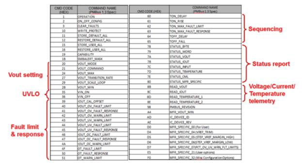
Figure 3. TPSM846C23 PMBus Commands Supported
