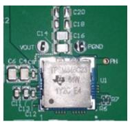
Figure 1. The 4.5V-15V, 35A TPSM846C23 PMBus Stackable Synchronous Buck Module
