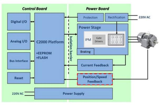
Figure 1. Basic Schematic of a Motor-drive System
