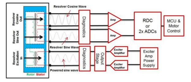
Figure 4. The Topology of Resolver Peripheral Circuits
