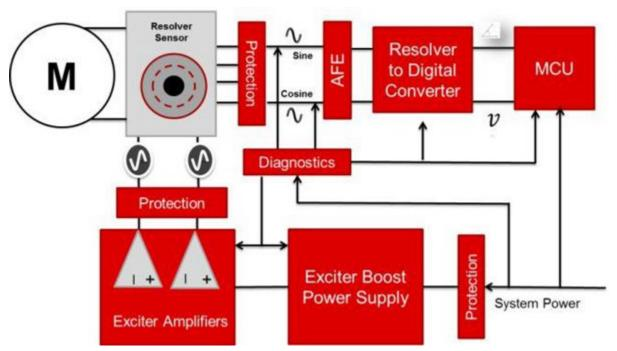
Figure 6. Resolver Interface Discrete Solution Topology
