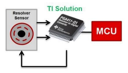
Figure 7. TI Resolver Interface Solution Topology
