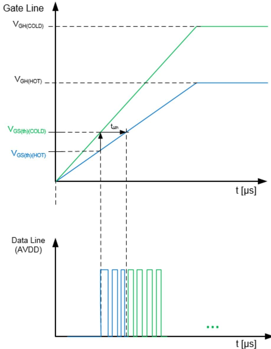
**Figure 3. Temperature Behavior TFT**
