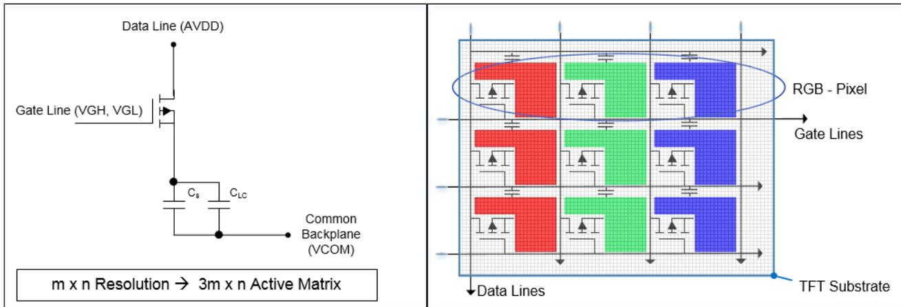
**Figure 2. Unit Pixel Structure + Equivalent Circuit**
