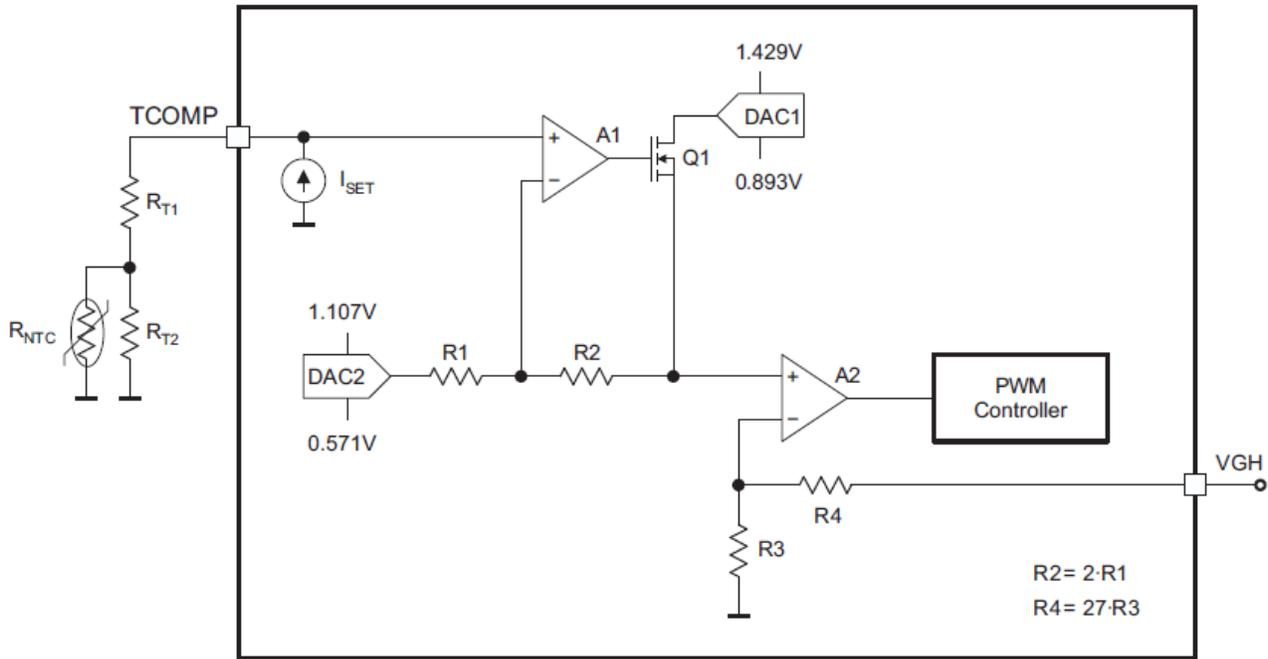
**Figure 5. Temperature Compensation Network TPS65642**
