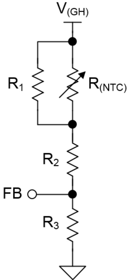
**Figure 4. Simple Compensation Network**
