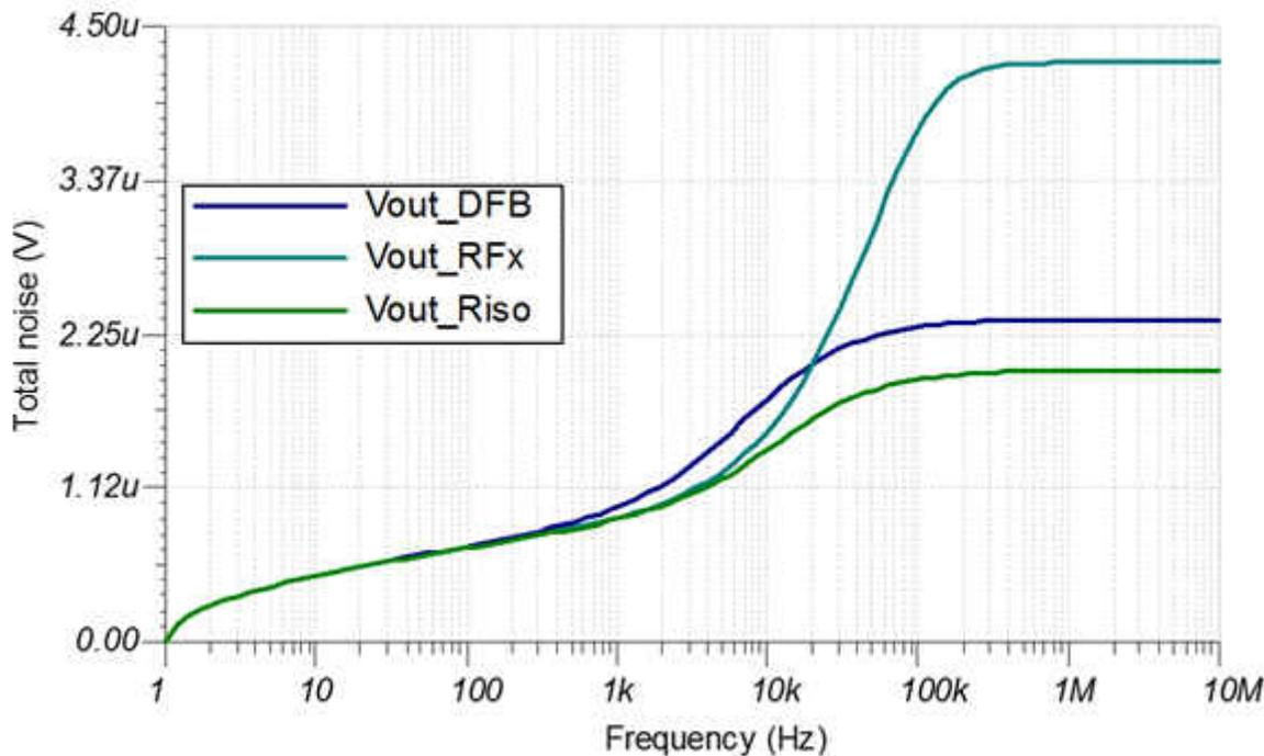
**Figure 5. Total output-noise comparison for the three compensation circuits**
