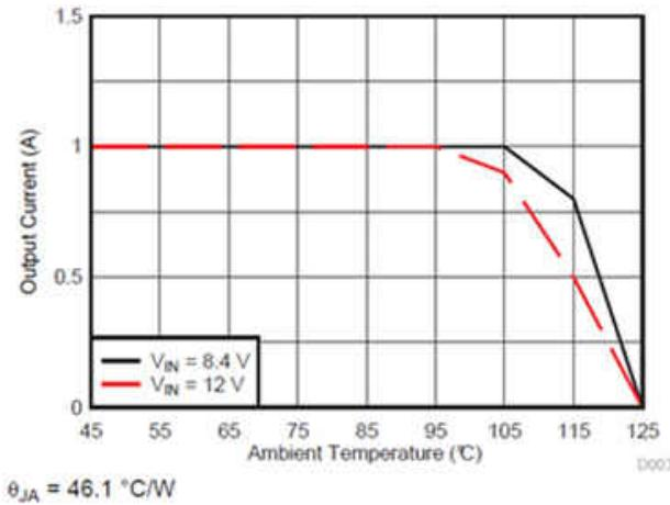
Figure 19. Thermal Derating,  $V_{\text{OUT}} = 5 \text{ V}$
