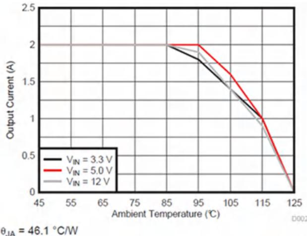
Figure 16. Thermal Derating,  $V_{OUT} = 1\text{ V}$
