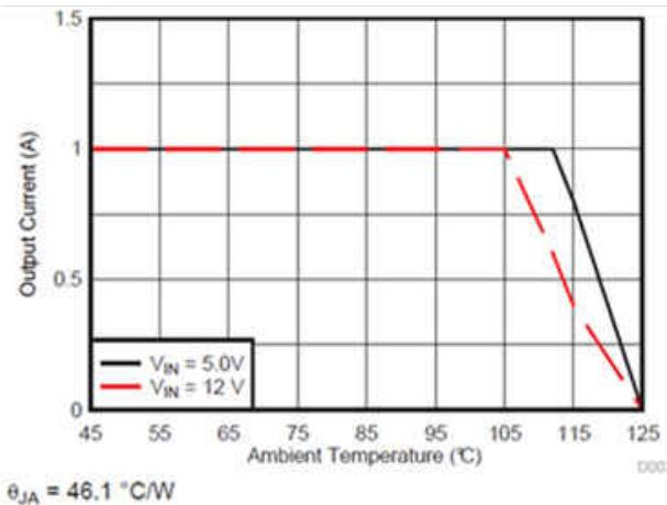
Figure 18. Thermal Derating,  $V_{\text{OUT}} = 3.3 \text{ V}$
