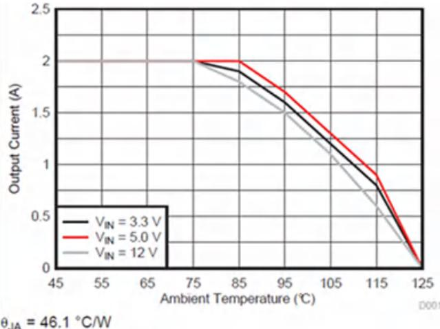
Figure 17. Thermal Derating,  $V_{OUT} = 1.8\text{ V}$
