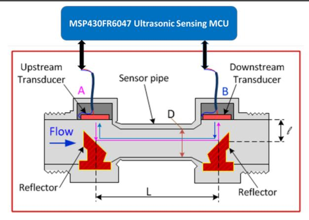
Figure 4. An MSP430 MCU Interface to Ultrasonic Flow Transducers in a Pipe
