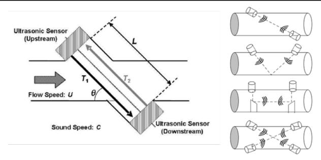
Figure 3. Examples of Ultrasonic Sensing for Flow Meters and Common Topologies for Positioning within a Pipe
