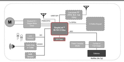
Figure 2. Smart Lock Diagram with SimpleLink Wi-Fi CC3220 Wireless Microcontroller
