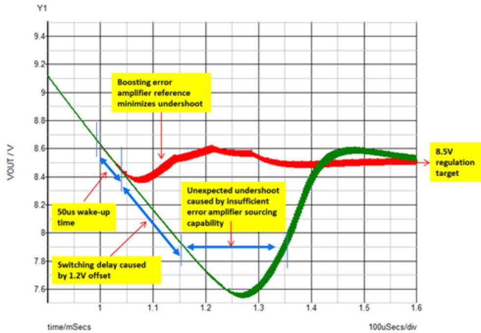
**Figure 2. Pre-boost Output Voltage During Battery Voltage Drop (a Traditional Boost Converter Shown in Green, the LM5150-Q1 Shown in Red)**
