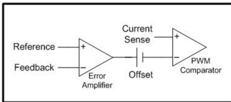
**Figure 1. Controller Block of a Boost Device**
