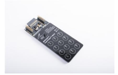
Figure 3. MSP430 CapTIvate Touch Keypad BoosterPack for the MSP430FR2522 MCU
