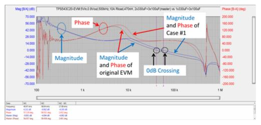
Figure 1. Bode Plot Comparison between Original Configurations versus Case No. 1
