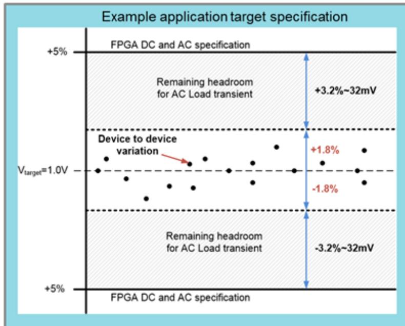
Figure 2. Target Specification with 5% Variation at a 1.0V Core Supply
